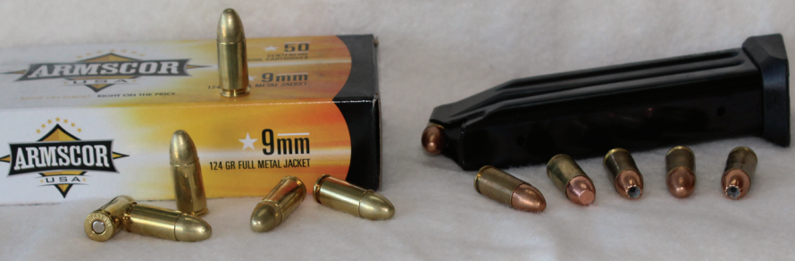
Typical loads for testing were one magazine with a mix of factory load FMJs and one magazine with a mix of reloads with FMJs, hollow points, and flat nose bullets in each caliber. Ones shown are 9mm.
